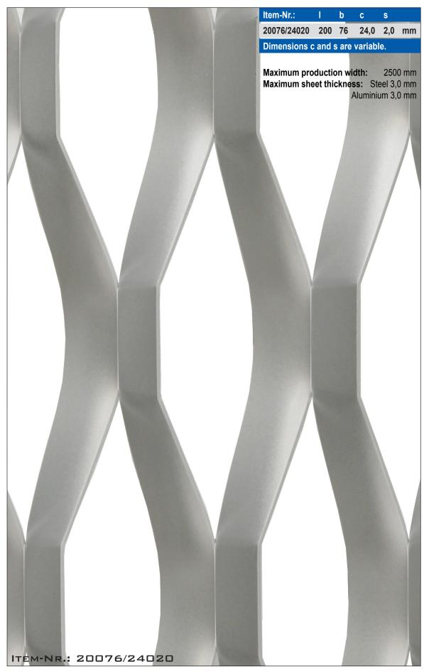
All meshes are available in different material thicknesses (s) and bond widths (c).
